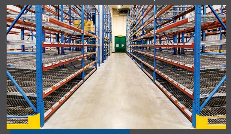
arton flow for pallet rack allows a warehouse or distribution center to utilize existing rack structure for more than just pallet positions. The integration of picking from carton flow alongside picking from pallets creates an efficient pick line layout that helps maximize picking efficiency.
