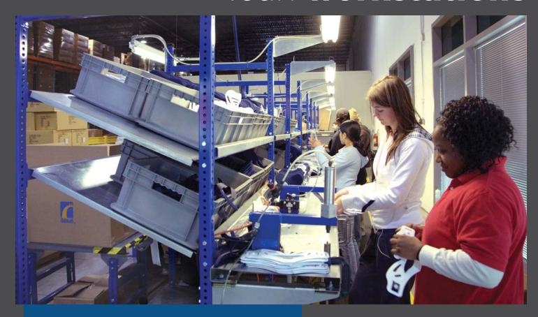
orkstations or sub assembly stations are a combination of a flow rack and a work surface where other operations are performed. Employees work faster, more accurately, and safer when they have an organized and functional workstation.
